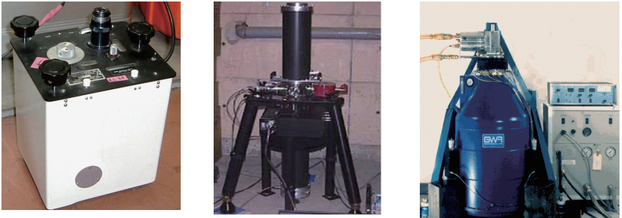
Fig. 1.1: Ground-based gravimeters. There are relative gravimeters (left), absolute gravimeters (AG) (middle) and superconducting gravimeters (SG) (right)
