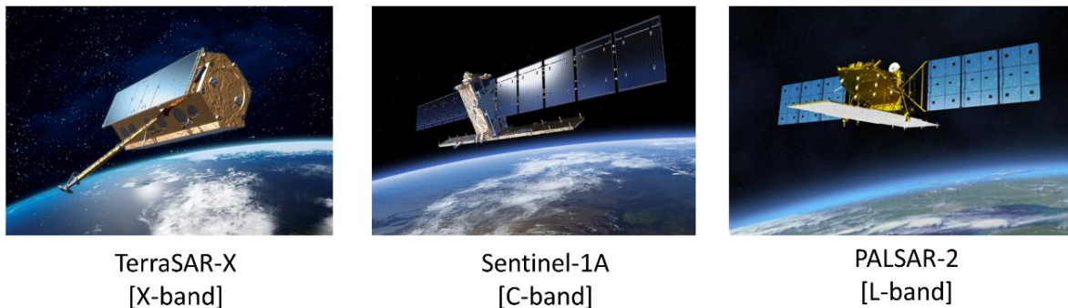
Figure 1.2 Pictures of SAR satellite, TerraSAR-X (Left, DLR, 2007 – ongoing, X-band [Wavelength: 3.1 cm]), Sentinel-1A (Center, ESA, 2014- ongoing, C-band [Wavelength: 5.6 cm]), PALSAR-2 (Right, JAXA, 2014 – ongoing, L-band [Wavelength: 23.6 cm])
