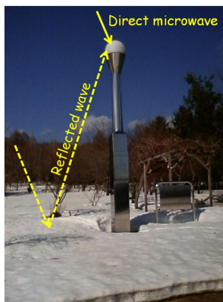
Figure. 1.2 : GEONET GPS station at the site 950128 in Fujino, Minami-ku, Sapporo-city.
